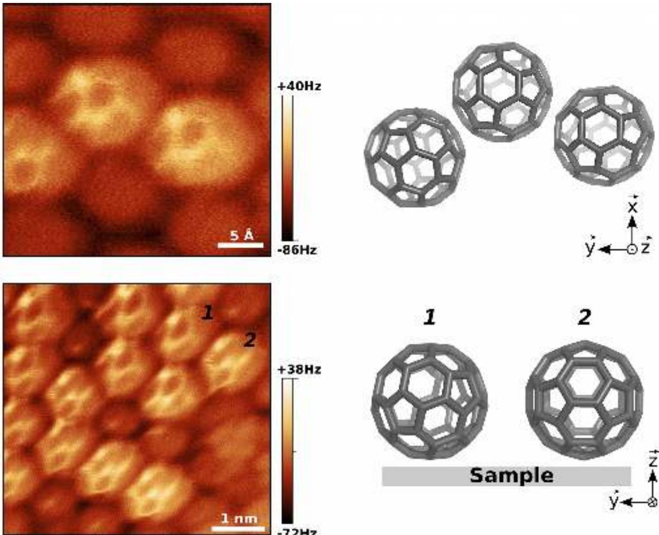
→ Constant-current AFM measurement (STM feedback I = 50 pA, V = 6 mV, A = 80 pm)
