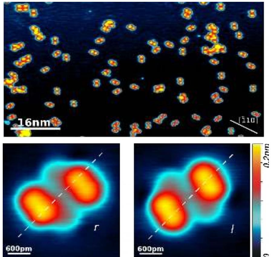
STM overview after deposition on the sample kept at 80K,
