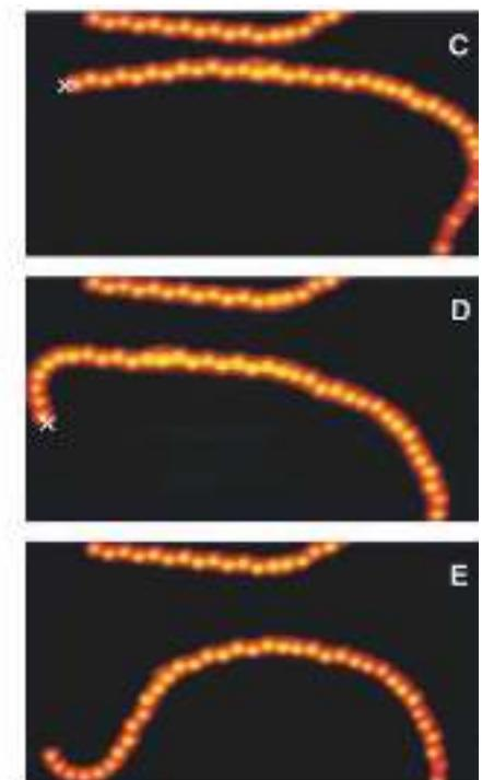
Fig. 2. Lifting a single molecular chain with the STM tip. (A) Scheme of the chain pulling procedure: After L. Lafferentz et al., Science 323, 1193 (2009).
