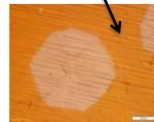
Optical images of graphene crystals on oxidized Cu substrate. Scale bar a) 50um b) 20 µm, c) 100 µm & d) 200 µm
