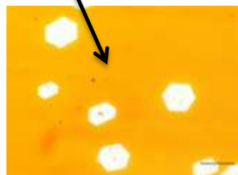
Optical images of graphene crystals on oxidized Cu substrate. Scale bar a) 50um b) 20 µm, c) 100 µm & d) 200 µm
