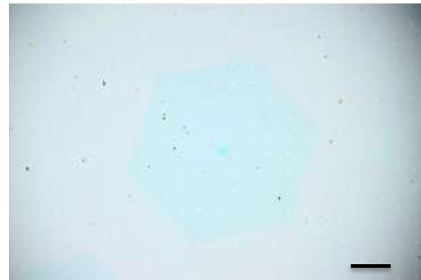
Optical Image of graphene after transfer to SiO 2 Scale bar: 400 μm
