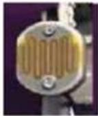
CDS Cell Resistive Light Sensor
