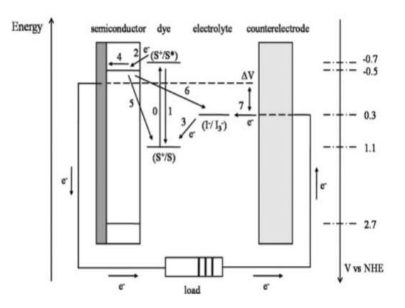
The process of electron transfer taking place at the oxide/dye/electrolyte interface
