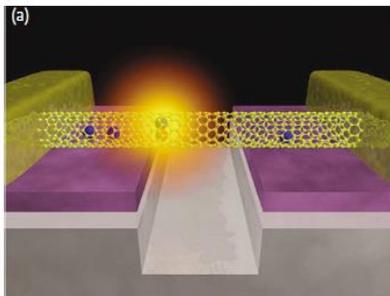
Place of recombination of electrons and holes controlled by  $V_g$
