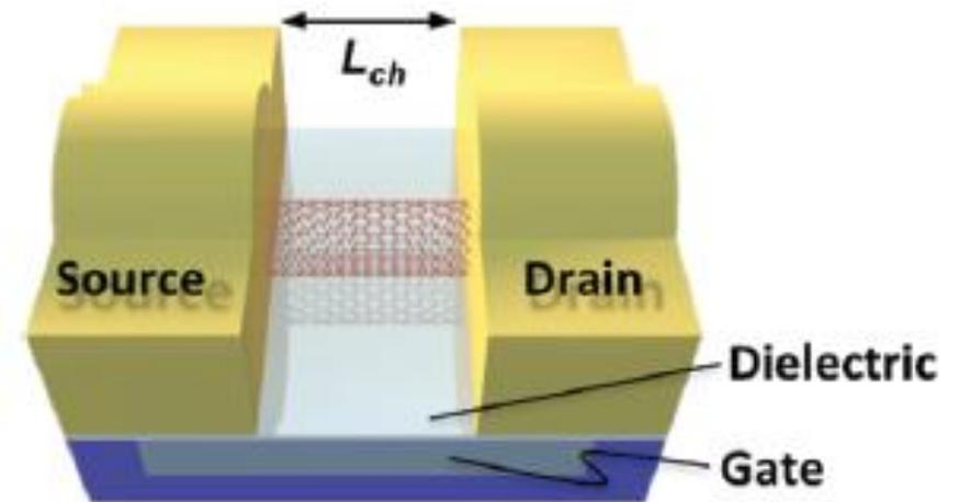
Electrodes on top of CNTs
