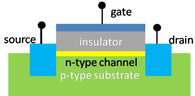
Gate voltage controls shape and conductivity of channel
