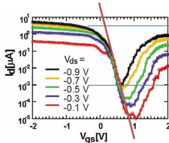
$$SS = \frac{1}{d \log_{10} I_d / d V_{gs}}$$
